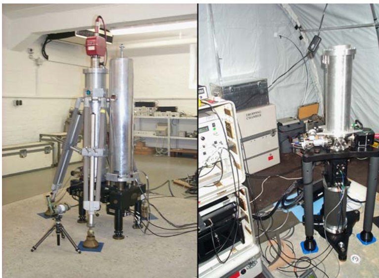
Figure 1: The two absolute gravimeters of the Leibniz Universität Hannover: left JILAg-3 employed from 1986 to 2000 (here reference measurements in Hannover), right FG5-220 operated since 2003 (tent measurements in Denmark)
